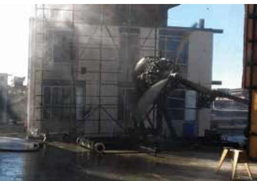
Dynamic Water Penetration Test of Mockup ©Clark Pacific 2013
